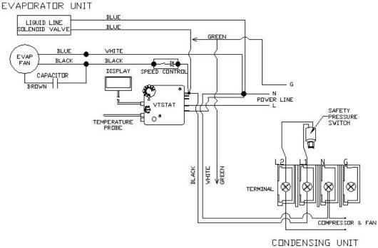
Fig. 2.2 VINO2500-4500SSR Electrical Wiring Diagram (VTSTAT)
